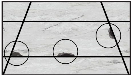
Fig.75 - Mortar displacement under edges and corners (risk of breaking with wheels or heavy loads).
