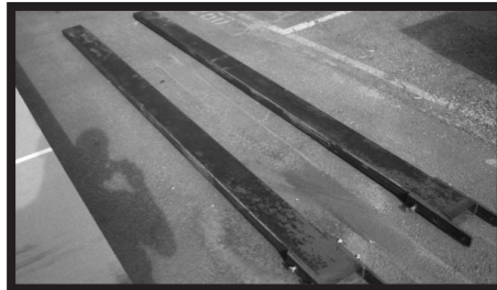
Fig.8 - We recommend using forks at least 84" long for maximum protection when handling from the short side. This will be necessary, since most US trucks do not allow for unloading and loading from the sides. 300 x 100 cm Florida Tile pallets are reinforced to allow maximum protection when being lifted from the short side and during handling by transporters.
