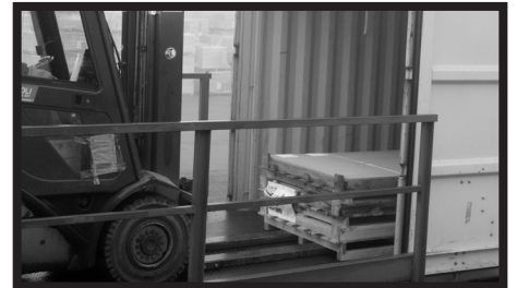
Fig.9 - Handling from long side with short forks is acceptable for short distances, but not ideal. We suggest this only for movement around warehouses or jobsites with minimal use. To move on pallets from their short side (i.e. when unloading trucks), you must use forks with a length of at least 84" to guarantee a sufficiently long supporting surface and to protect the pallet and its contents.
